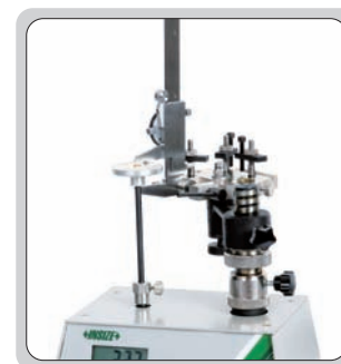
check the measuring force of calipers
