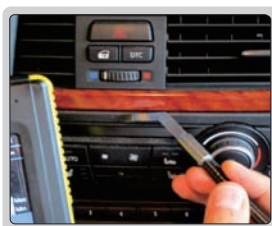
measuring gaps on the car dashboard
