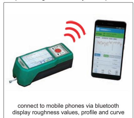
operate roughness tester by mobile phones
