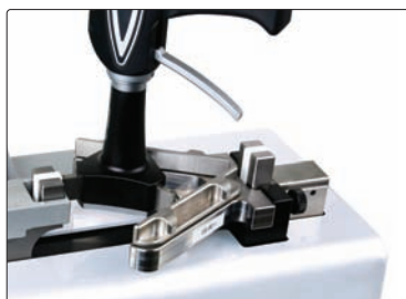
zero setting and calibration of three-point internal micrometers
