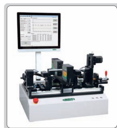
clamping workpieces by V-type bench center
