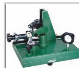
check the effect of lateral force on accuracy of test indicators (half round gauge block is needed)
