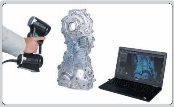
high-speed scanning: 26 crossed blue laser lines
