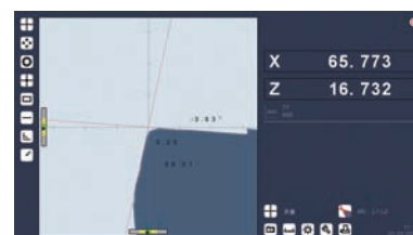
dynamic crosshair automatically adjusting as X and Z axis move, and the cutting tools can be quickly measured through the dynamic crosshair
