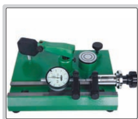
inspect accuracy of dial indicators (range 0-25mm)
