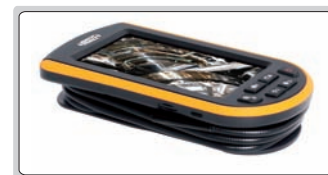
cable can be wrapped around the main unit
