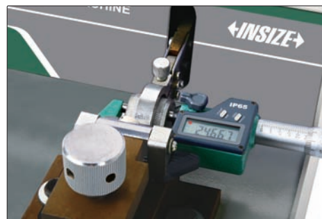
lapping measuring surfaces of outside micrometer
