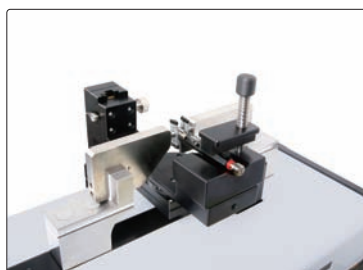
measuring thread plug gauges (manual mode)
