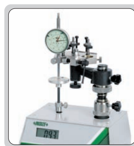
check the measuring force of dial indicators
