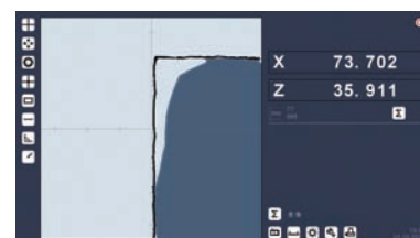
scanning the maximum profile of cutting tools
