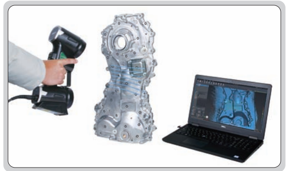
precision scanning: 7 parallel blue laser lines
